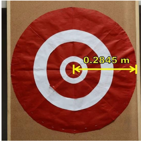
Figure 7: Landing area design with white concentric circles. Radius of the largest red circle measures 0.2845m.
