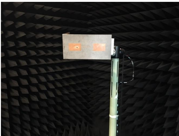
Figure 11: Measurement setup of bend-array structure (side-view)
