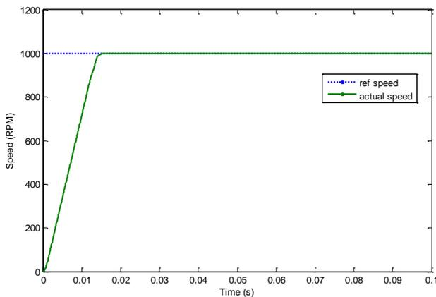
Figure 7: Speed Response with ref 1000 RPM
