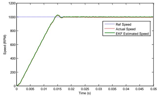
Figure 9: Actual and Estimated speed (EKF) responses with PI Controller
