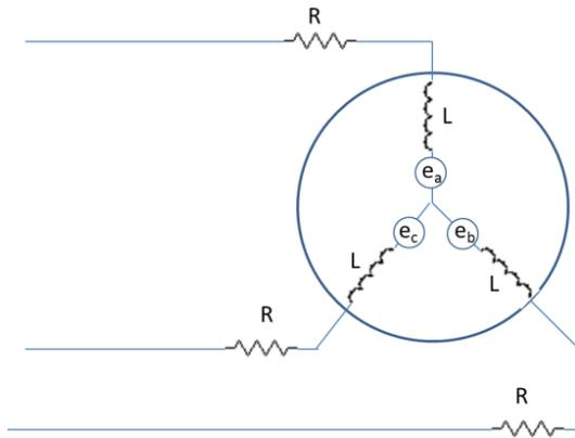
Figure 1: Equivalent Circuit of BLDC Motor
