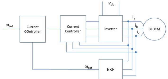
Figure 2: System Configuration
