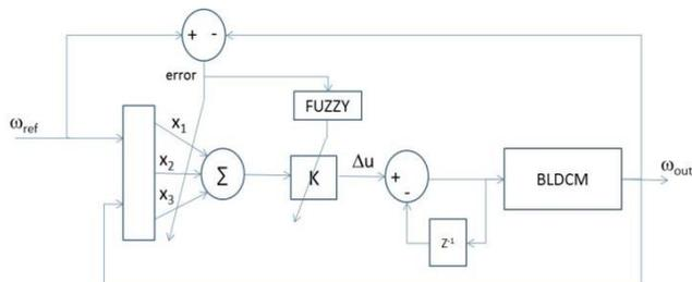
Figure 3: The structure of the single neuron-Fuzzy controller for BLDCM
