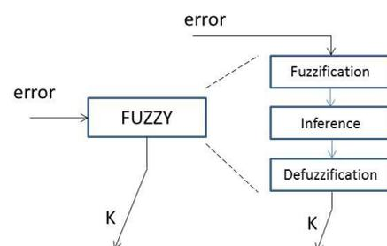
Figure 4: The Structure of Fuzzy Logic Controller
