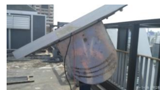
Figure 4: Actual Tilting Mechanism
