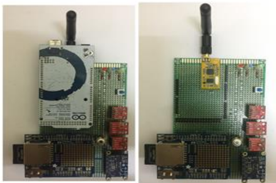
Figure 2: Breakout Board on Donut Prototyping Board
