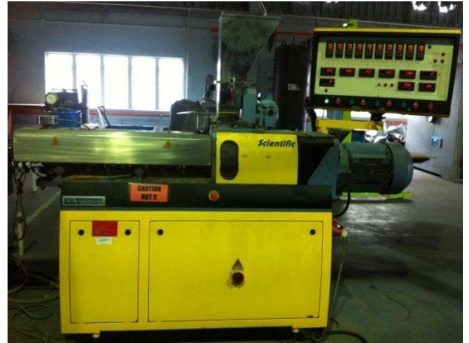
Figure 2: Hot mixer for WPC method
