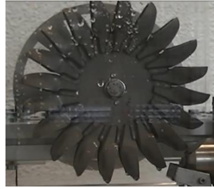
Figure 4: Pelton turbine enclosed in a chamber
