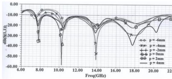
Figure 7: Return loss with varying position of coupled patch on top of substrate 'p'
