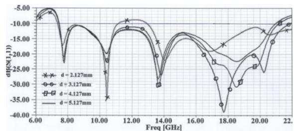
Figure 6: Return loss with varying parasitic patches 'd'
