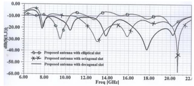
Figure 10: Return loss with varying ground plane and slot shape
