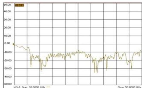
Figure 12: Return loss (measured) 10MHz to 50GHz
