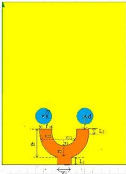
Figure 2: The antenna substrate back view with dimensions
