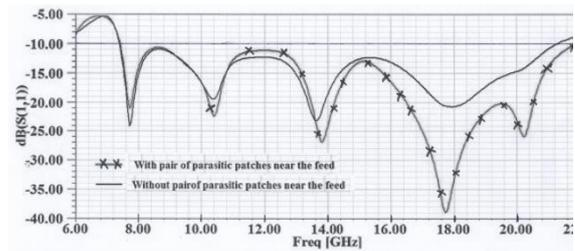
Figure 4: Return loss with and without circular parasitic patches
