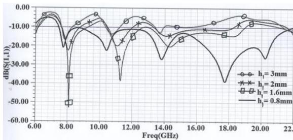
Figure 8: Return loss with varying substrate thickness 'h<sub>1</sub>'
