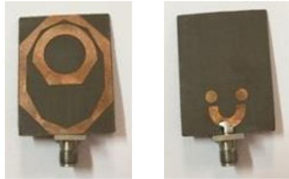
Figure 3: Fabricated antenna-top and bottom view
