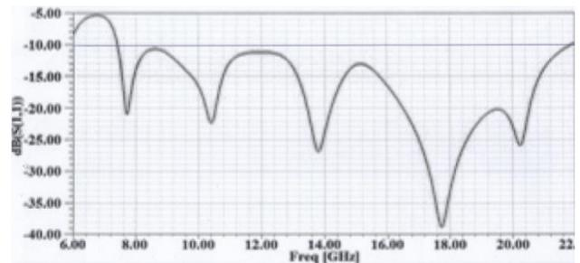
Figure 11: Return loss of antenna (simulated)
