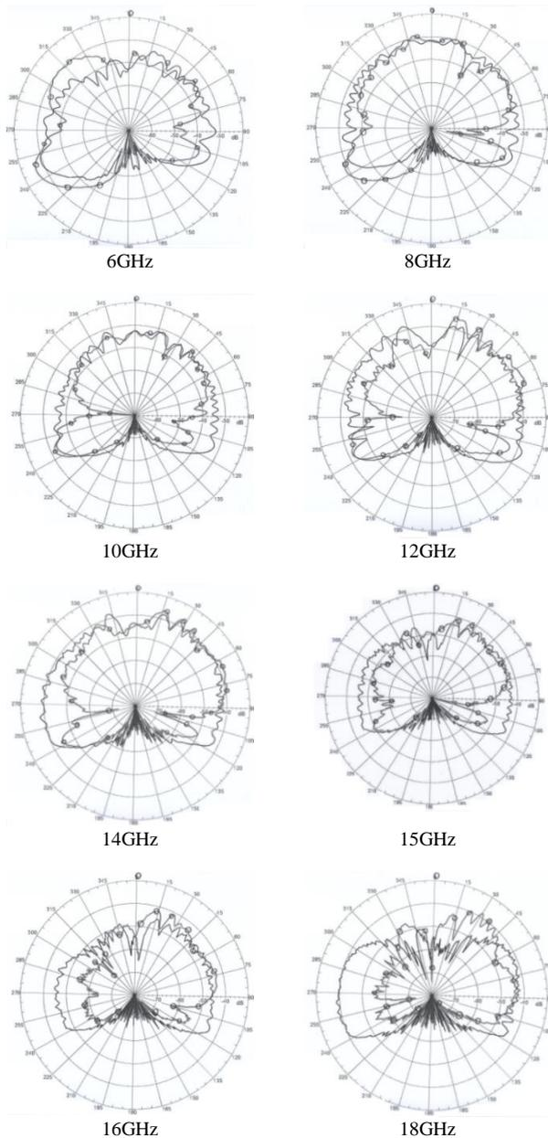
Figure 13: Radiation patterns (measured)
