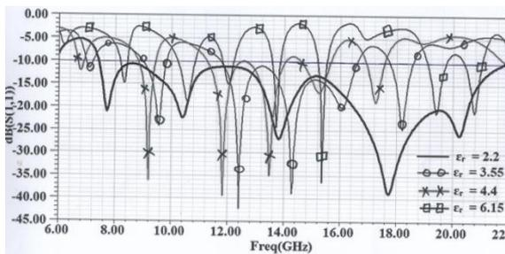
Figure 9: Return loss with varying dielectric constant of substrate 'ε<sub>r</sub>'
