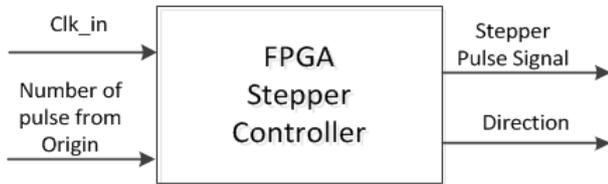
Figure 1: Controller input and output
