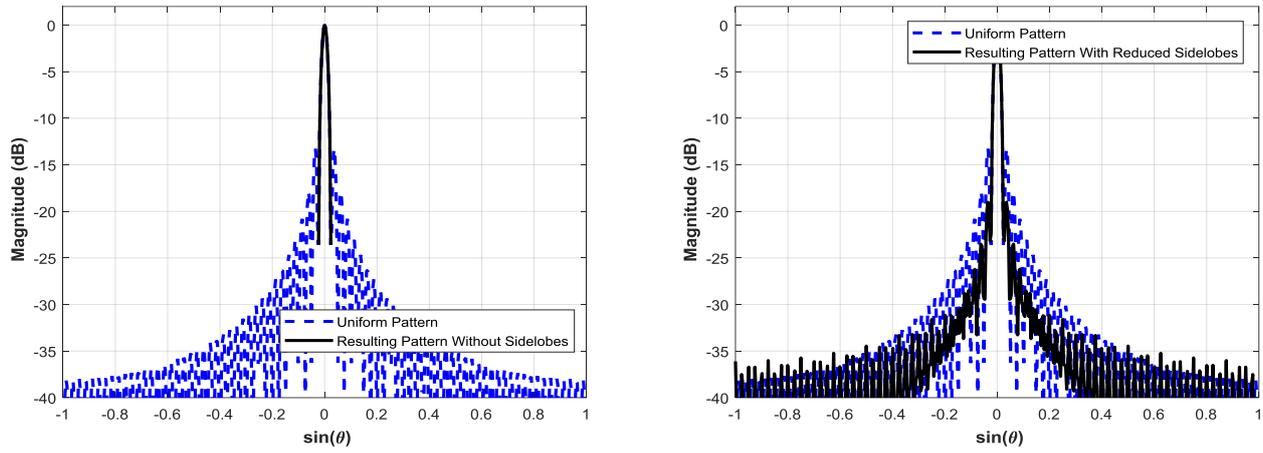
Figure 6: The resulting patterns for  $N=80$  and  $K=512$ . Exact case (left) and Approximate case (right).
