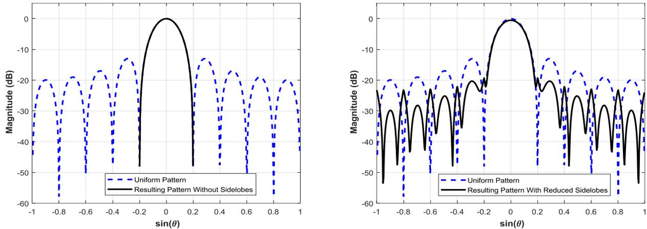
Figure 4: The resulting patterns for N=10 and K=512. Exact case (left) and Approximate case (right).
