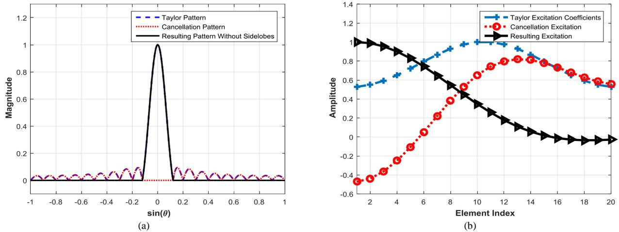
Figure 9: (a) The resulting patterns for Taylor array and N=20, (b) the corresponding element excitations.
