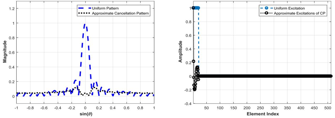
Figure 2: The Approximate Cancellation Pattern (left) and its Corresponding Element Excitations (right) For  $N=20$  and  $K=512$ .
