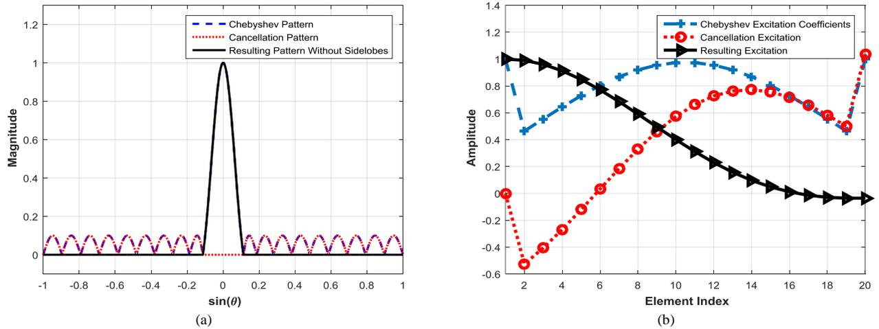
Figure 8: (a) The resulting patterns for Chebyshev array and  $N=20$ , (b) the corresponding element excitations.
