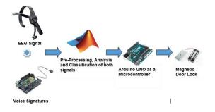
Figure 7: Research block diagram
