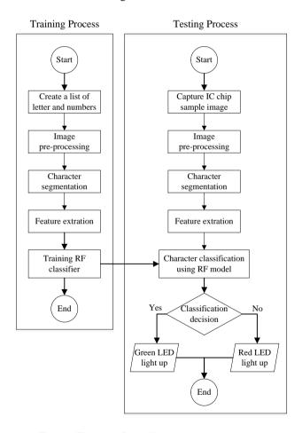
Figure 1: Flowchart of embedded character recognition system
