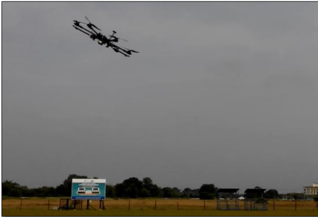
Figure 2: Hexarotor flying in sinewave form for 5 minutes
