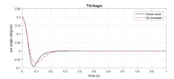
Figure 15: Tilt angle for increasing the Derivative gain,  $K_D$ .
