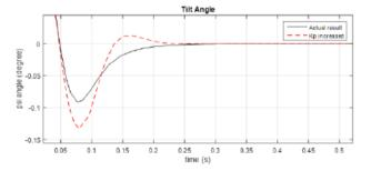
Figure 13: Overshoot for increasing the Integral gain, K<sub>1</sub>.
