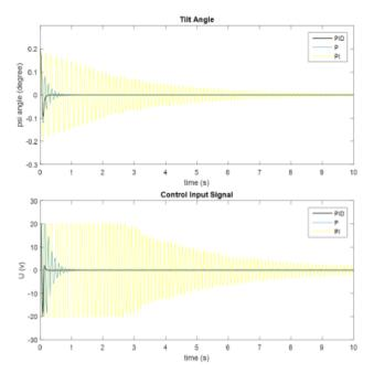
Figure 8: The tilt angle and control input signal (U) of P, PI and PID controller.
