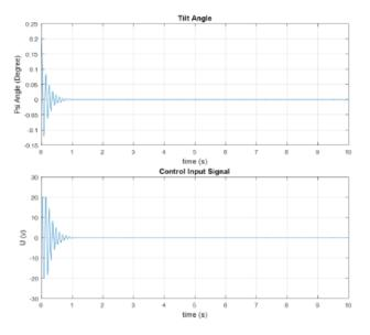
Figure 6: The tilt angle and control input signal (U) of P controller
