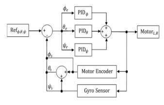
Figure 2: The PID controller diagram.
