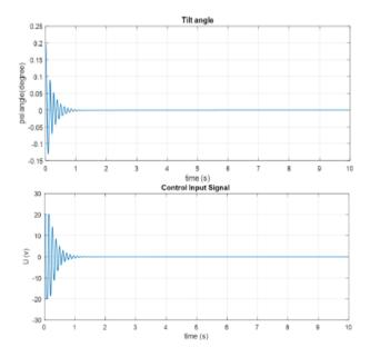
Figure 3: The tilt angle and control input signal (U) of the system using PID tuner tuning method.
