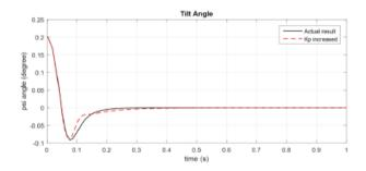
Figure 9: Tilt angle after increase the gain P
