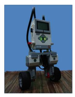
Figure 1: Two-wheeled balancing EV3 LEGO robot.
