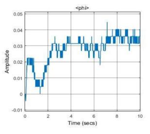
Figure 20: Hardware real-time tilt angle response.
