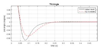
Figure 16: Overshoot for increasing the Derivative gain,  $K_D$ .
