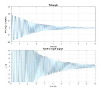
Figure 7: The tilt angle and control input signal (U) of the system using PID trial and error tuning method.
