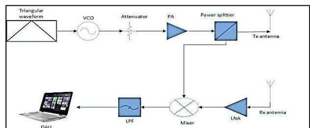
Figure 1: FMCW radar block diagram [7]
