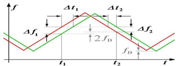
Figure 4: Linear triangular waveform [7]
