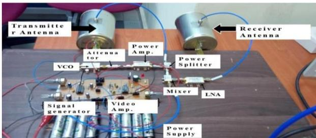
Figure 6: Assembled FMCW Radar [7], [9]
