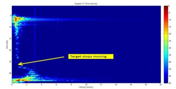
Figure 7: Measured velocity of the target movement
