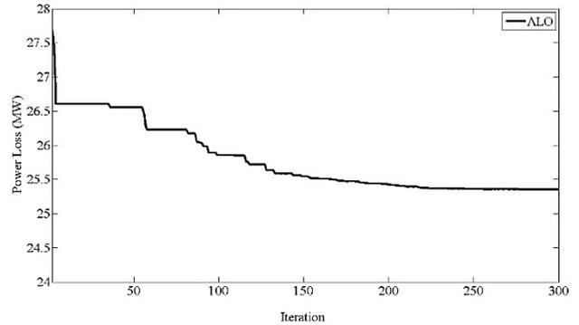
Figure 4: Convergence performance of ALO for power loss minimization
