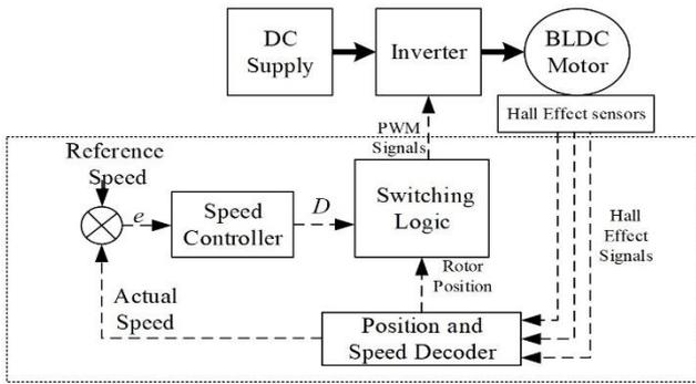
Figure 1: Speed Controller of BLDC Motor
