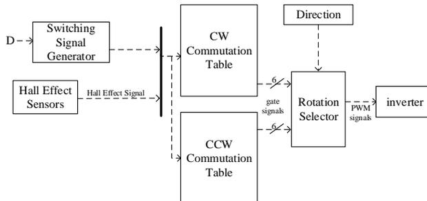
Figure 5: Direct commutation switching scheme controller
