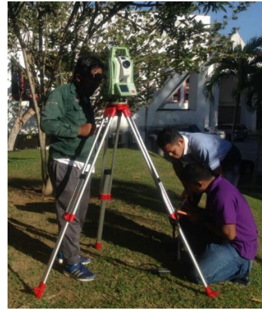
Figure 6: JUPEM officers equipped with Theodolite observing the sun, in order to determine the true north direction
