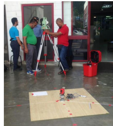
Figure 7: The direction of true north, which was transferred point-by-point to the semi-open space, and the marked difference of true north direction, which was done by a prototype, was observed
