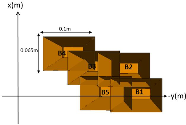
Figure 8: Feed horn arrangement
