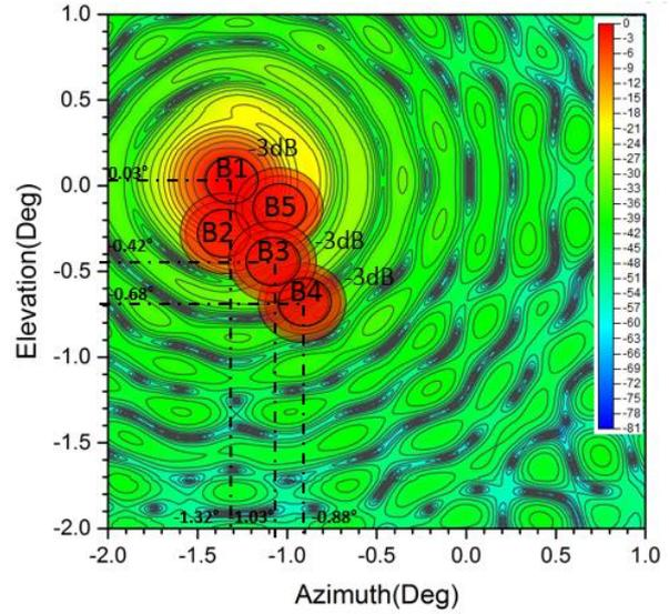
Figure 10: Two-dimensional radiation pattern view for Peninsular Malaysia
