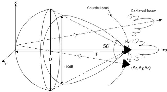
Figure 3: Parabolic reflector antenna with feed horns
