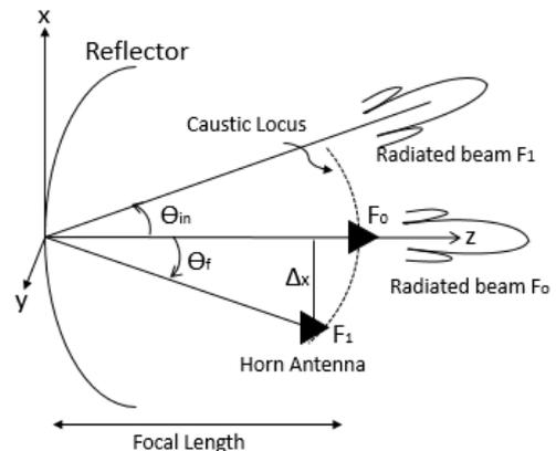
Figure 5: Relation of feed points and radiated beams
