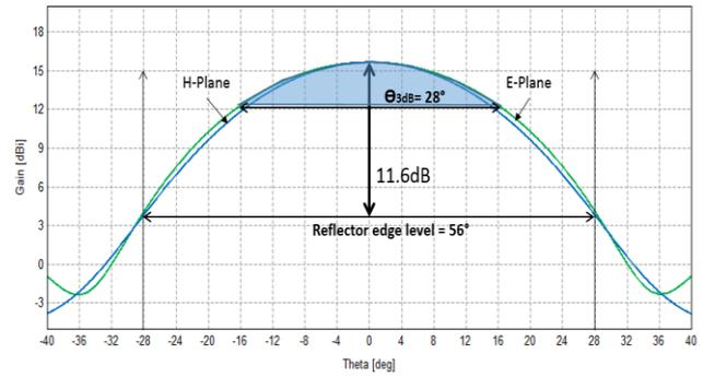
Figure 7: Pyramidal horn radiation pattern
