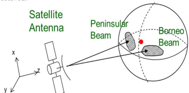
Figure 2: Malaysia beam from satellite point-of-view
