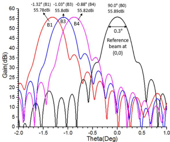
Figure 9: One-dimensional radiation pattern of beam on Line A with reference beam at (0,0)
