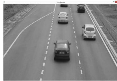
Figure 2: Effect of grayscale conversion and Gaussian blur operation
