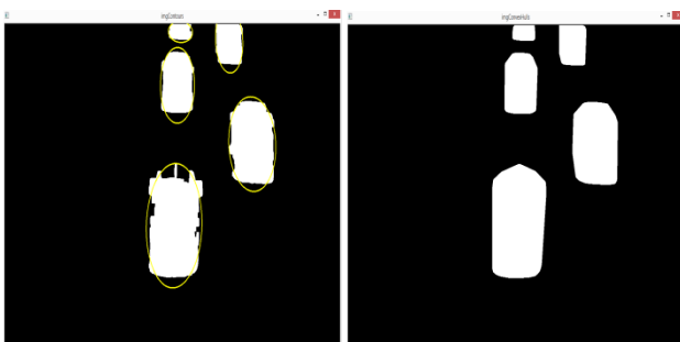
Figure 4: Effect of (a) contour tracing (b) convex hull generation
