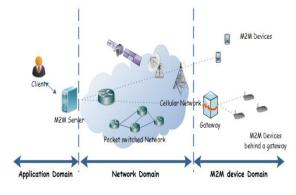
Figure 2: General Architecture of an M2M Application [4]
