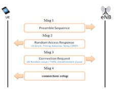
Figure 3: RA procedure signaling
