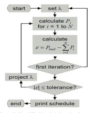
Figure 2: Simplified Lambda Iteration Process
