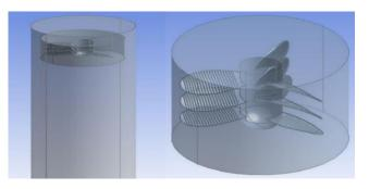
Figure 1: Submerged fan with transparent column
