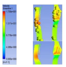
Figure 3: Velocity profile of submerged fan
