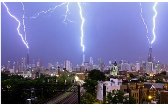
Figure 3: Simultaneous lightning strikes to three tall buildings in Chicago [4]
