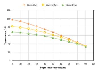
Figure 8: Temperature generated for different electrode ratio with  $\sigma = 1.09$  S/m
