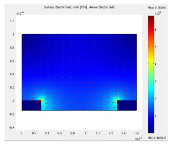
Figure 6: Gradient of electric field for electrode with width:gap ratio of 60µm:180µm
