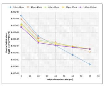
Figure 4: Electric field gradient distribution for different 1:1(width:gap) electrode ratio
