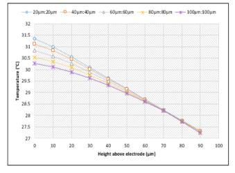
Figure 7: Temperature generated for 1:1 (width:gap) electrode ratio with  $\sigma$ = 0.0575 S/m
