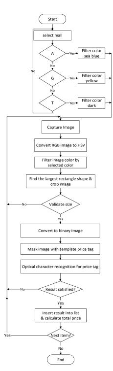
Figure 2: Image processing engine pipeline
