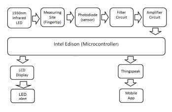
Figure 1: Overall structure of project
