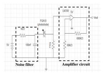
Figure 2: Filter and amplifier circuit
