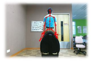
Figure 4: RGB with skeletal tracking image of rider on Equicizer
