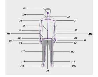
Figure 2: 25 skeletal joints relative to the human body that can be detected by Kinect for Windows V2 (adapted from [10])
