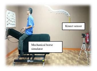
Figure 3: Setup for data collection
