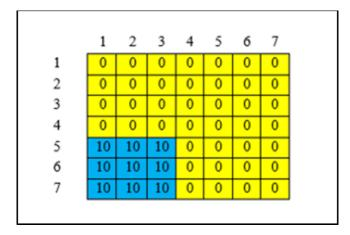
Figure 2: Example of attenuation coefficient representing the presence of the object.
