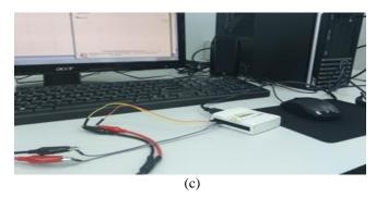
Figure 2: (a) Electrode placement on the subject (b) BMA-400 Bioamplifier and ISO-Z amplifier (c) National Instrument USB-6009 connected to computer and the input from bio-amplifier
