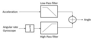
Figure 2: Block diagram of complementary filter
