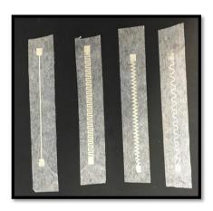
Figure 3: Screen-printed electrodes on Micropore
