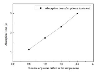
Figure 5: Effect of the distance of plasma tube orifice to fabric sample against time of water absorption after APPJ treatment for 5 seconds.
