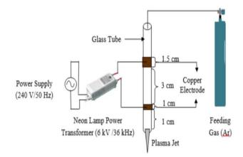
Figure 1: Configuration of atmospheric pressure plasma needle jet using copper electrodes and neon transformer power source. Argon gas flow is fixed at 50 L/min.
