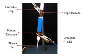
Figure 2: Photo image of atmospheric pressure plasma needle jet. Length of plasma jet is about 2 cm from the tube orifice.
