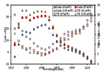
Figure 6: Gain and noise figure of the double-pass Zr-EDF by using optical circulator as the reflector for different pump power with input signal fixed at -30 dBm
