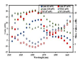
Figure 7: Gain and noise figure of the double-pass Zr-EDF by using optical circulator as the reflector for different pump power with input signal fixed at -10 dBm
