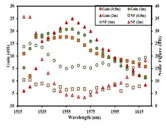
Figure 5: Gain and noise figure of the double-pass Zr-EDF by using optical circulator as the reflector for different lengths of gain medium with input signal fixed at -10 dBm
