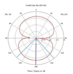
Figure 5: The radiation pattern for the Tubular type.
