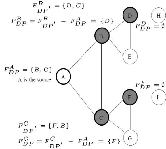
Figure 5: Failure of dominant pruning algorithm
