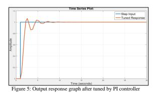
Figure 7 shows the system tuned via proportional integral
