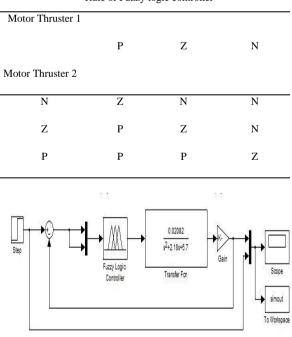
Figure 11: Simulink block diagram for AUV system
