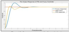
Figure 15: Output response graph after optimization
