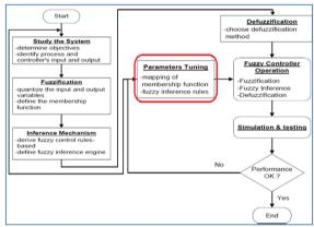
Figure 3: Flow Chart of Design Methodology of FLCs.
