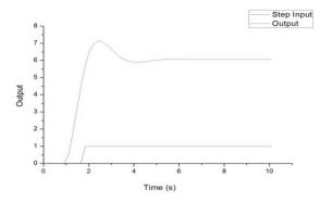
Figure 12: Output response after implemented gain block
