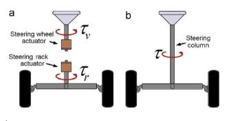
Figure 1: (a) VSBW (b) Conventional Steering System
