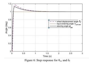
The front wheel displacement angle can track the steering wheel angle with zero steady state error. But the percentage overshoot, %OS is higher than  $\theta_{sw}$  which is 19%. Both responses have an identical settling time,  $T_s$  which is less than 1 second.
