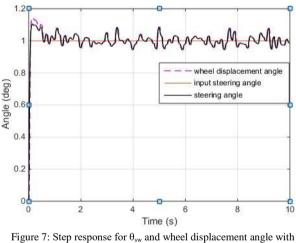
Figure 7: Step response for  $\theta_{sw}$  and wheel displacement angle with disturbance.
