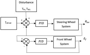
Figure 4: Block diagram of VSBW system
