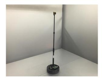
Figure 3: SP360 camera mounted on iRobot Creat2
