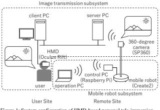
Figure 1: System configuration of HMD-based personal tele-immersion system
