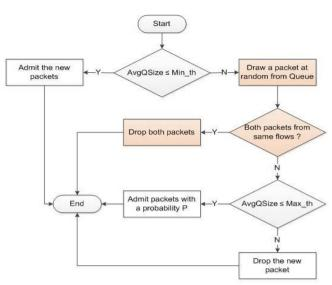
Figure 2: CHOKe Algorithm Flowchart
