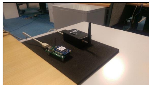
Figure 6: Sniffer node (Left) placed near the base station (Right) for better packet interception
