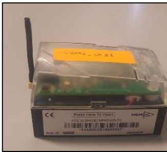
Figure 3: MicaZ Sensor Node (Radio Module with Sensor Board)
