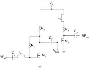
Figure 13: Schematic of the proposed UWB PA [23].
