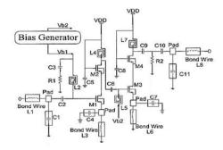
Figure 7: Schematic of the proposed UWB PA [7].
