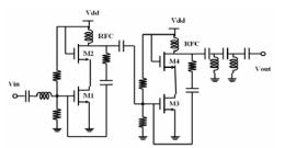
Figure 9: Schematic of proposed UWB PA [8].
