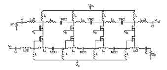
Figure 2: Schematic of the distributed amplifier topology with a wide bandpass artificial transmission line [2].
