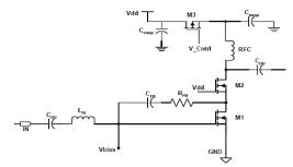
Figure 4: Schematic of the input stage of PA [3].
