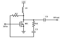
Figure 8: Shunt-shunt feedback and resistive feedback at the output stage
