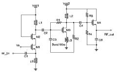
Figure 10: Schematic of the proposed UWB PA [9].
