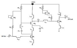
Figure 19: Schematic of the proposed UWB PA [15].
