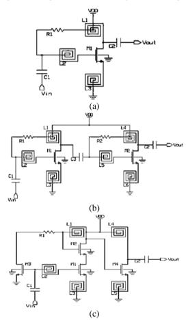
Figure 15: (a) Single-stage UWB PA (b)Double-stage cascaded UWB PA (c)Double-stage cascoded PA [20]
