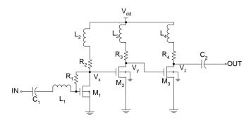
Figure 20: Schematic of the proposed UWB PA [16]
