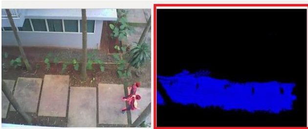
a. Vision detects changes b. Accumulated pixel changes
