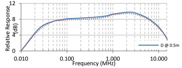
Figure 6: Relative response of square aluminum tube (Item D)
