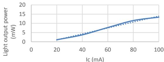
Figure 12: Radiometric output power for different IRLED forward currents.
