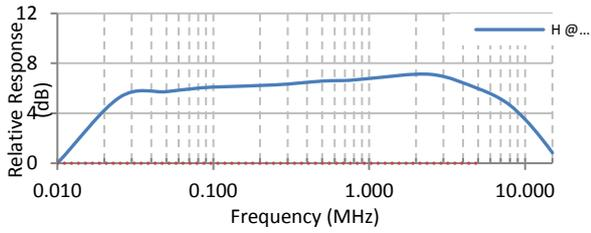
Figure 10: Relative response of square mild steel tube (Item H)
