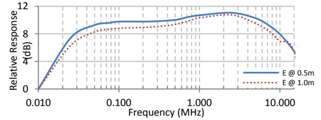
Figure 7: Relative response of square aluminum tube (Item E)
