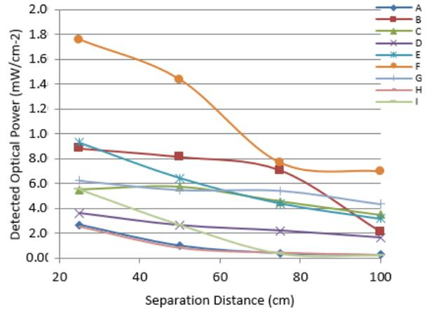
Figure 14: Received optical power plotted against separation distance.
