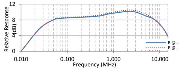
Figure 4: Relative response of circular plastic tube (Item B)
