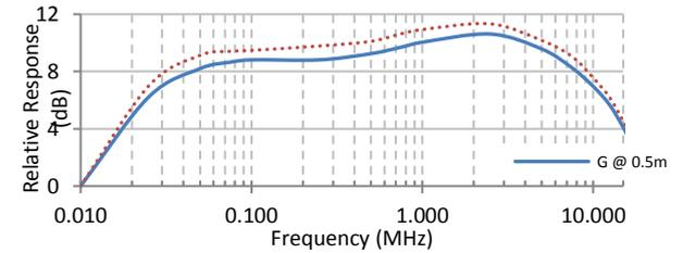
Figure 9: Relative response of circular galvanized aluminum tube (Item G)
