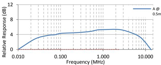
Figure 3: Relative response of circular cardboard tube (Item A)
