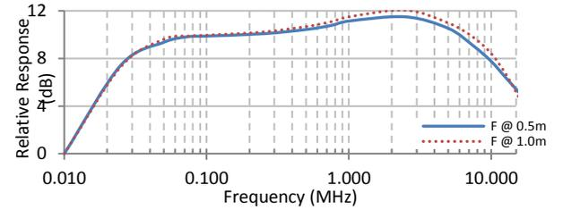
Figure 8: Relative response of circular aluminum tube (Item F)
