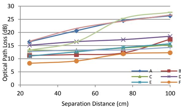
Figure 16: LOS optical path loss at different separation distances
