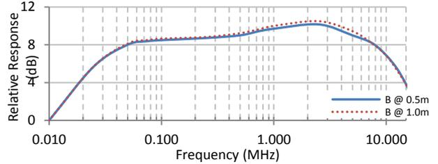
Figure 5: Relative response of circular mild steel tube (Item C)
