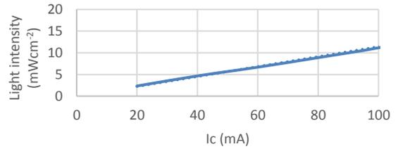
Figure 13: Photometric output power for different IRLED forward currents.
