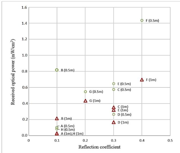
Figure 15: Received optical power plotted against reflection coefficient at 0.5 metre and 1 meter range.
