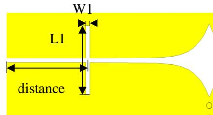
Figure 4: Geometry of Rectangular slot
