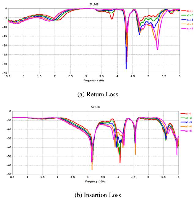
Figure 6: Parametric study of S-parameter for width of rectangular slot
