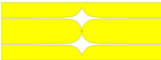
Figure 2: Basic structure of 1x4 Power Combiner
