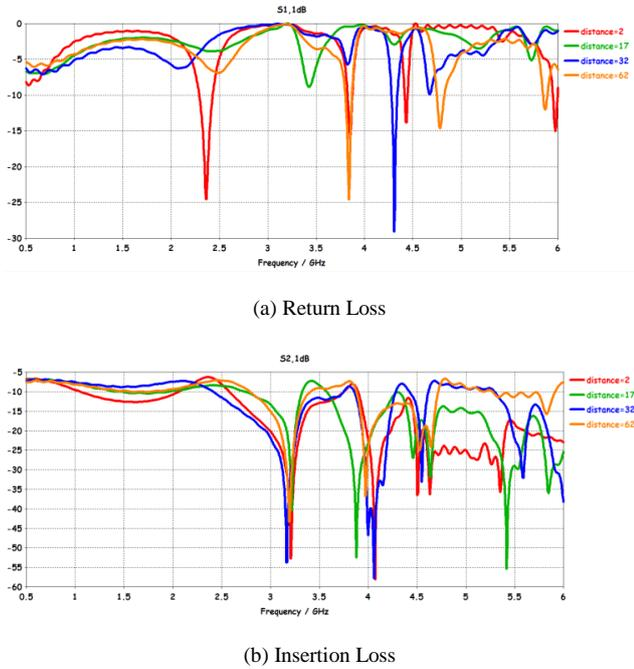
Figure 5: Parametric study of S-parameter for distance of rectangular slot
