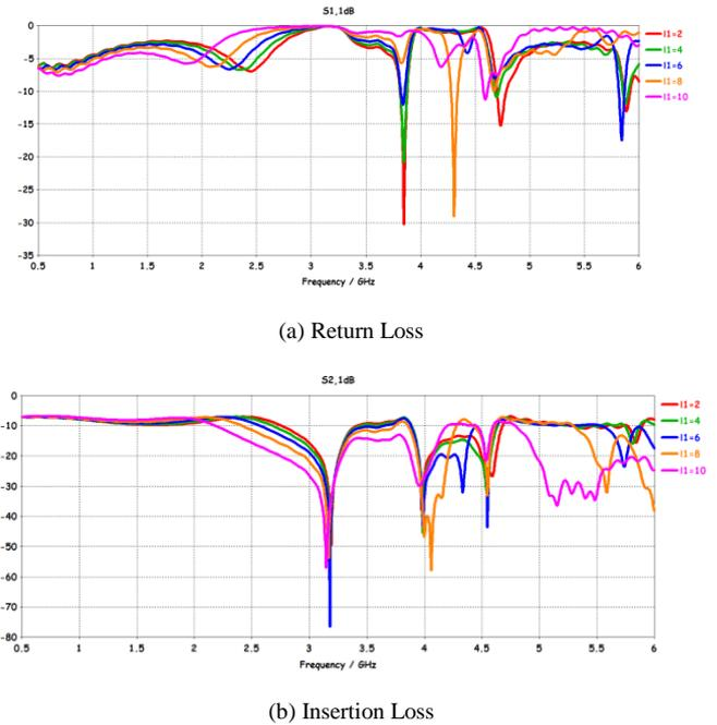
Figure 7: Parametric study of S-parameter for rectangular slot
