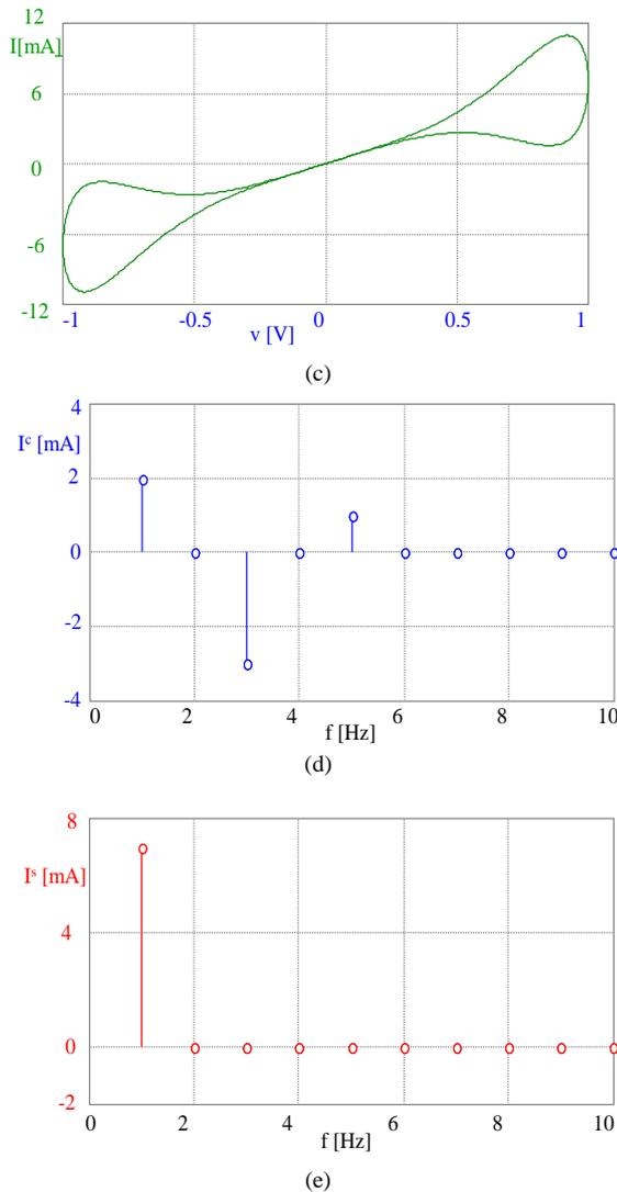
Figure 2: SPICE simulation of the model from Figure 1: (a) voltage and current waveforms, (b) memductance vs time, (c) type-II pinched hysteresis loop with 3<sup>rd</sup>-order touching at  $v - i$  origin, (d), (e) cosine and sine spectral terms of current
