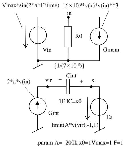
Figure 1: Schematic for SPICE model of memristive system described by Equation (16) and (25)
