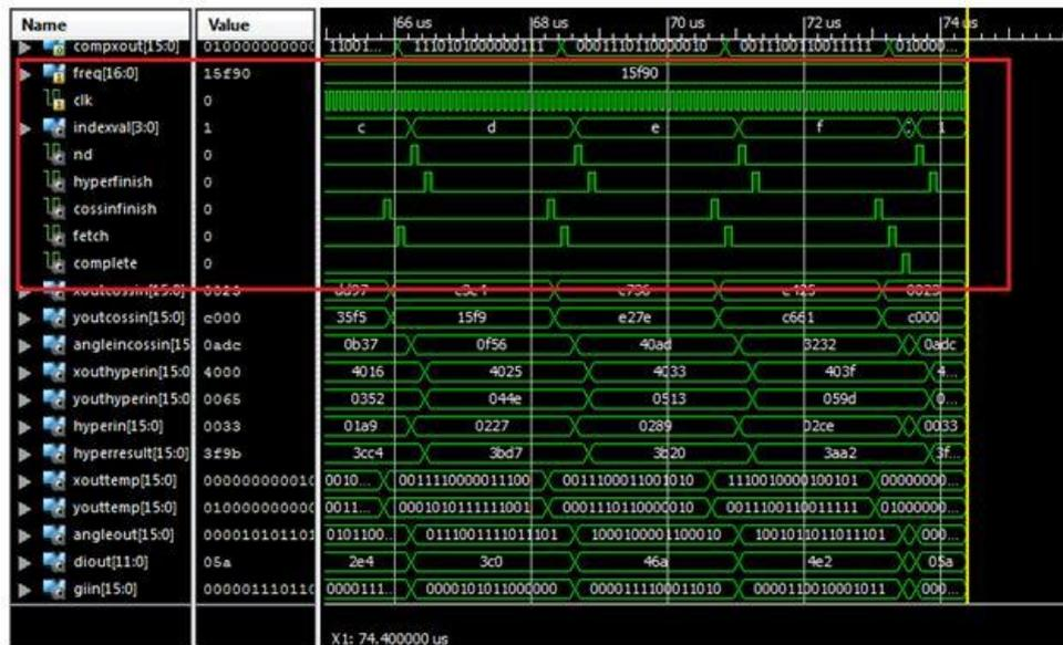
Figure 6: Timing Relation of Various Signals
