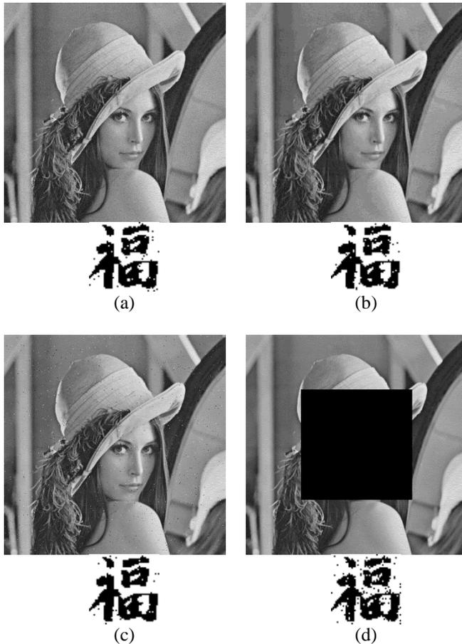
Figure 8: Attacked watermarked Lena images and watermark recovery: (a) Gaussian Noise 0.001, (b) JPEG compression, (c) Salt and Pepper 0.005, (d) Cropping centred 25%.
