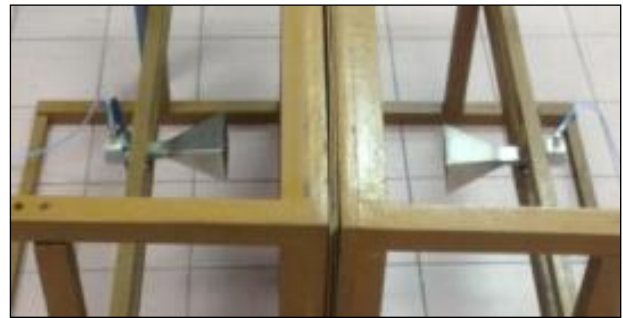
Figure 5: Free space dielectric measurement setup
