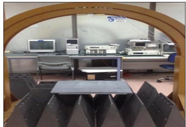
Figure 6: Free space arch measurement setup
