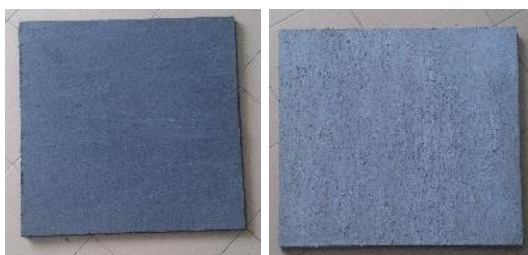
Figure 4: Plywood applied with (a) carbon (b) palm ash
