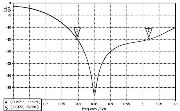
Figure 4: Return Loss of a dipole patch antenna
