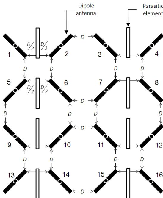
Figure 2: A *star* configuration of 4x4-array dipole antenna
